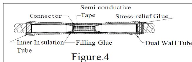
**6. Heat up inner insulation tube and dual wall tube.**
