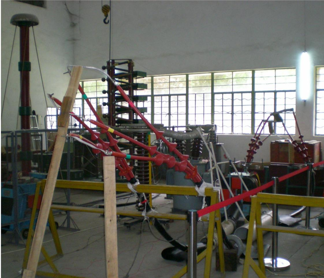
Complete test set-up during impulse voltage test at high temperature
