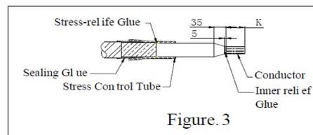
**3. Peel off the insulation layer and fix up stress control tube.**
